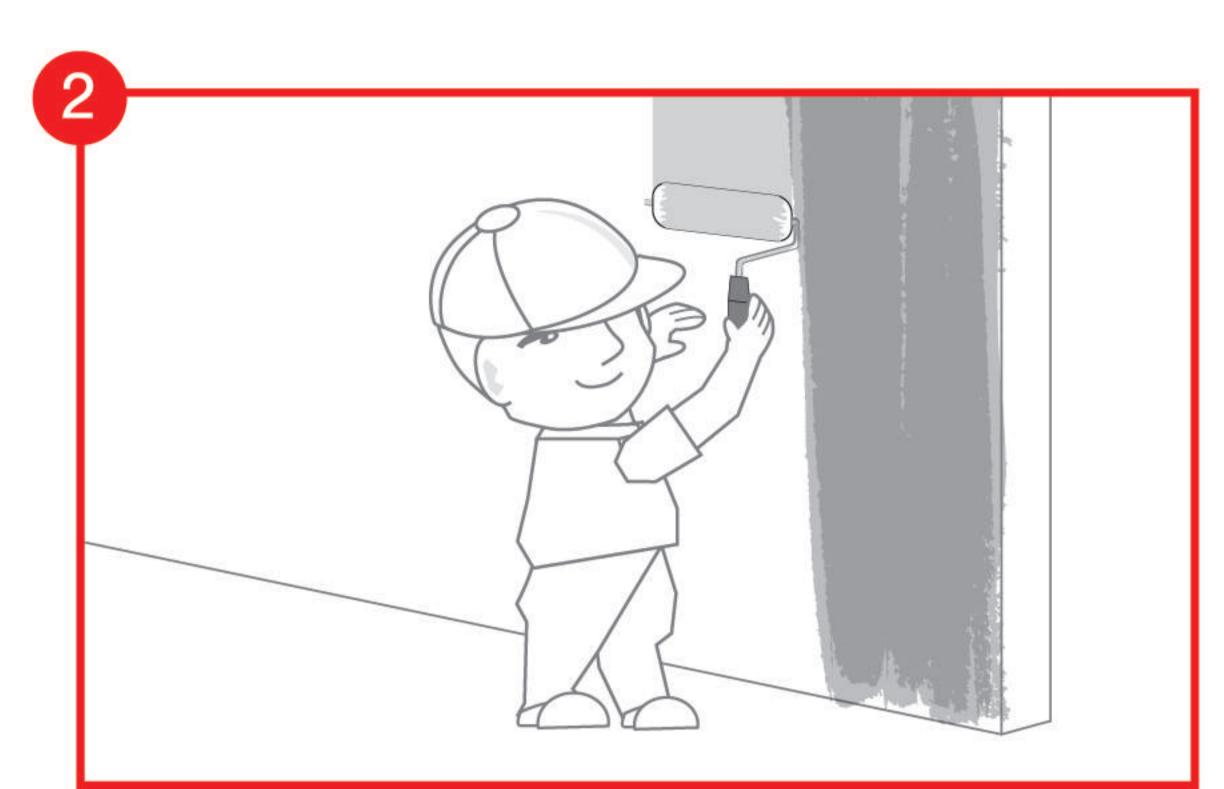
Prepare the SCG Smartboard surface by cleaning and painting contact primer over the old surface. Then leave to dry.
