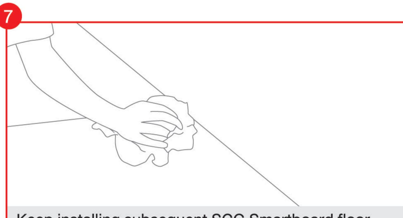
Keep installing subsequent SCG Smartboard floor panels until the work is finish. Then clean the floor surface to be free of dust and oil stains by using a damp cloth.
