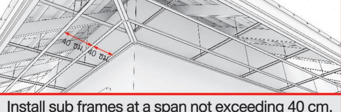
Install sub frames at a span not exceeding 40 cm.
